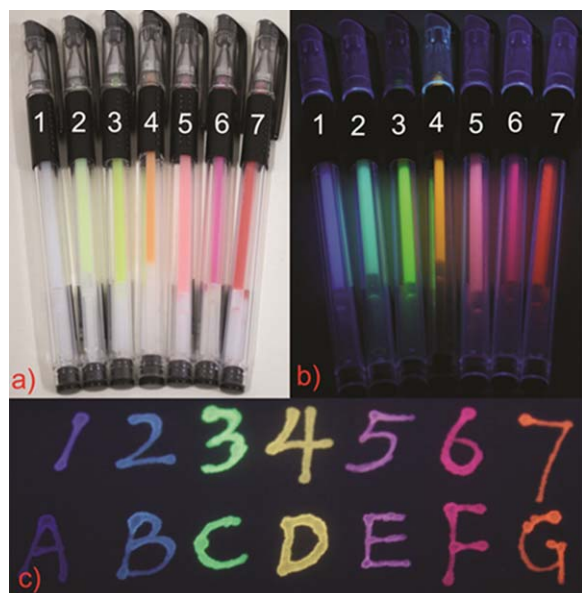
Figure 8. (a) Multicolor fluorescent pens obtained via using different MFPNs inks (1: NP-A1; 2: NP-B1; 3: NP-B3; 4: NP-C7; 5: NP-C1; 6: NP-C2; 7: NP-C5). (b) Photograph recorded of fluorescent pens illuminated by a portable UV lamp. (c) Photograph recorded of multicolor numbers and letters via writing on paper via different pens (from 1 to 7, or A to G) (illuminated by a portable UV lamp). [Color figure can be viewed in the online issue, which is available at wileyonlinelibrary.com .]
